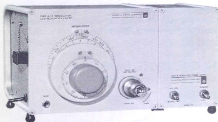
Type 1362 UHF Oscillator with Type 1267-B Regulated Power Supply.
